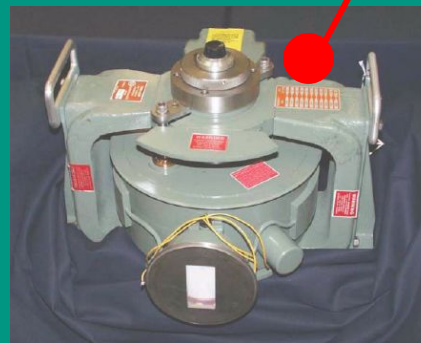
CPI 1143B 3 MW S-Band Magnetron
